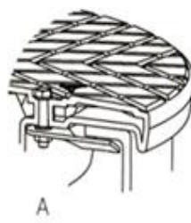
A Safety latch opened B Safety latch closed
